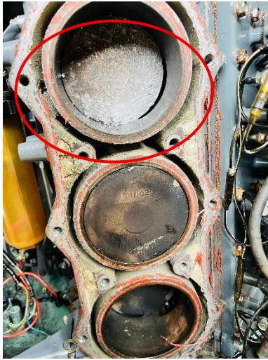
Figure 5. Damaged Cylinder Sleeves and Pistons
