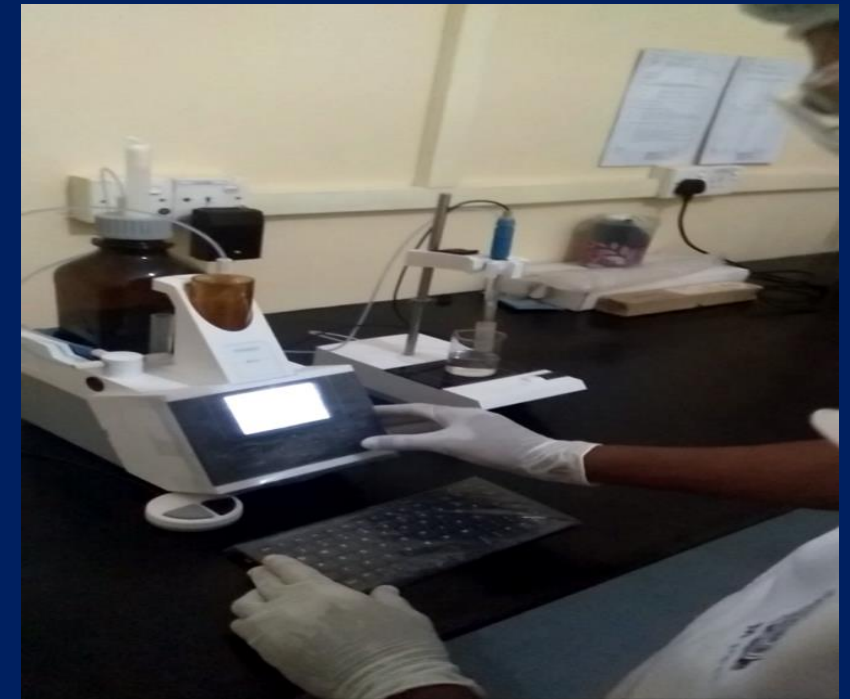
Total Base Number Testing as per - ASTM D 2896/4739
