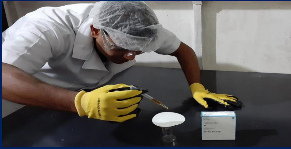
Drop Test (Blotter Paper) as per - ASTM D 7899
