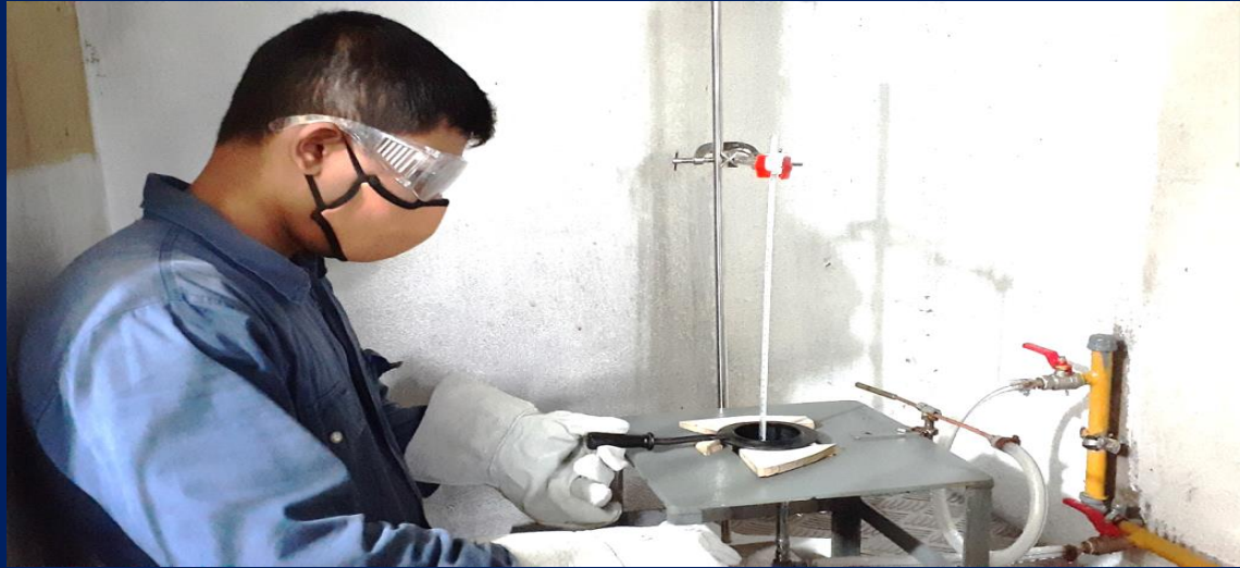
Flash Point Tester As per – ASTM D 92
