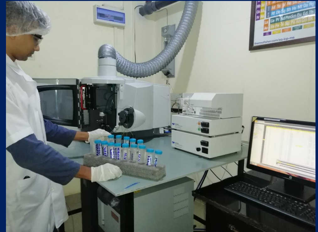
iCAP 7200 ICP-OES Radial Oil Spectrometer, USA
