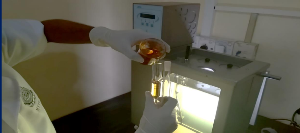
Kinematic Viscosity Testing as per - ASTM D 445
