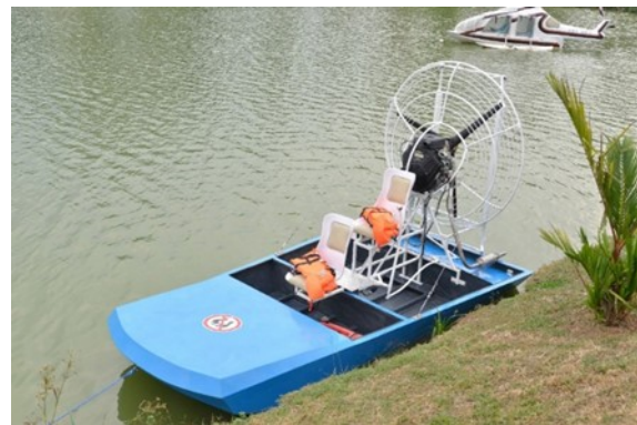
Figure 4: Seating arrangement of airboat
