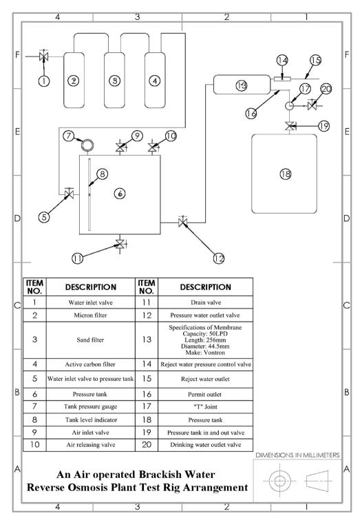
Figure 4. Schematic of air operated BWRO plant.
