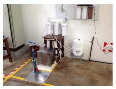
Figure 2. Air operated domestic use brackish water reverse osmosis plant.
