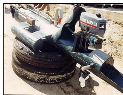
Figure 2. Explosive Laden Floating Device
