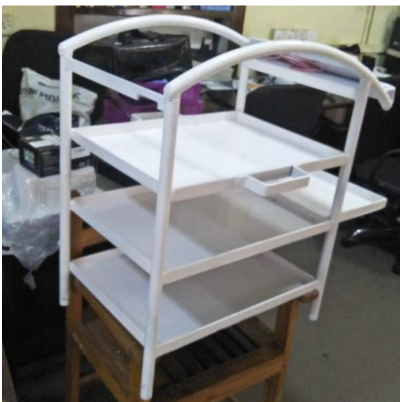
Fig 12. Aluminum structure with 3 trays.
