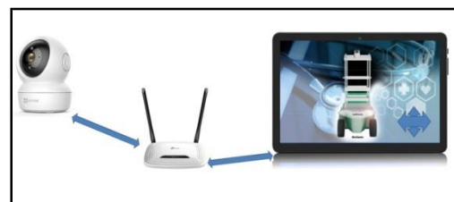
Fig 13. Basic connection diagram of camera, router and tablet.
