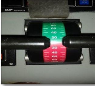
Fig. 7. Back Up And Indication Unit
