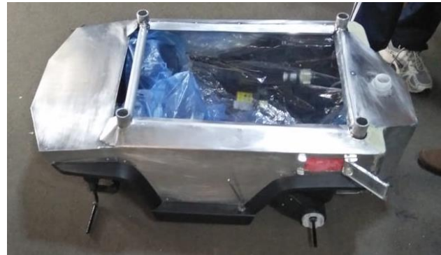
Fig 5. Aluminum body design of rover.
